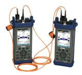
A matched combination of Optical Light Sources and Optical Power Meters to create a loss test set or kit for particular applications.
